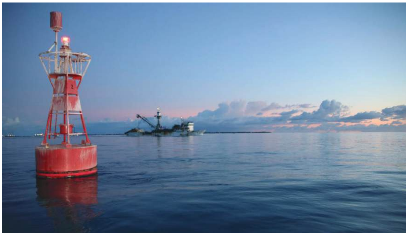
IALA AtoN (aid to navigation): These buoys are part of the IALA Maritime Buoyage System, used globally to ensure safe navigation.
