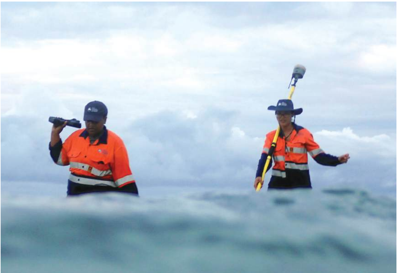
SPC's Ocean Science Technicians carrying out a field survey along Fiji's Coral Coast to collect topography points and extract data from pressure sensors or tide wave recorders.
