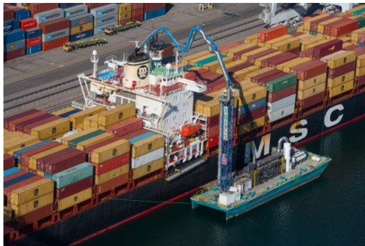
Figure 4-4 Typical Emission Capture System (Picture courtesy of AMECS website)
