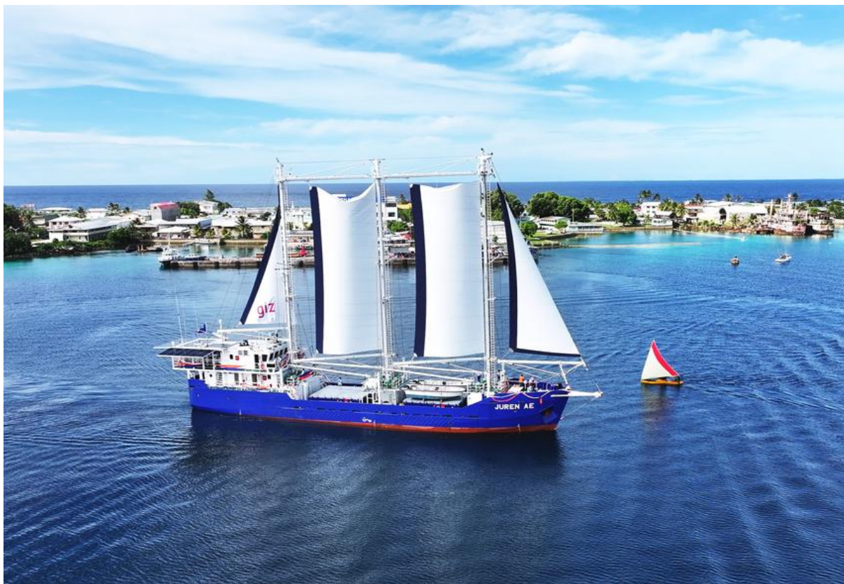
Caption: The Wind-hybrid cargo ship SV Juren Ae under sail in the Marshall Islands (Image: Chewy Lin / GIZ LCST)
