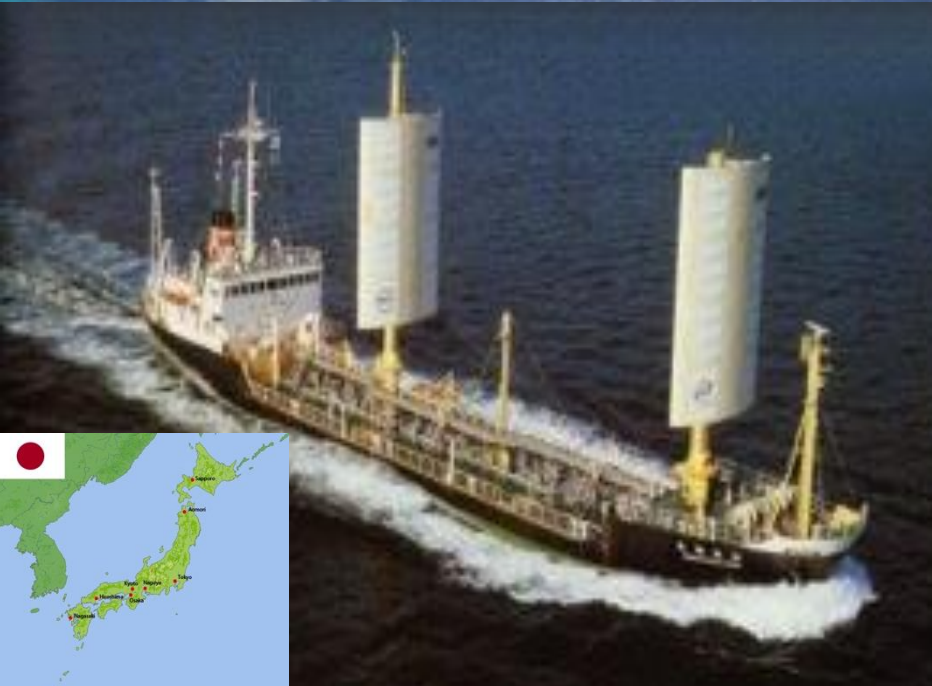
SAILING-DEISEL-POWERED ISLAND TRADING VESSEL FOR CARGO & PASSENGERS 91'0A, 86'4" DEEP WL, 21'
