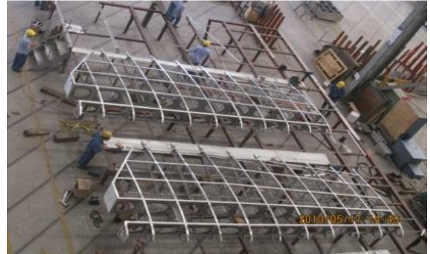
OCIUS Lotus Wing Solar Sails under construction at Afai Shipyard Guangzhou, China
