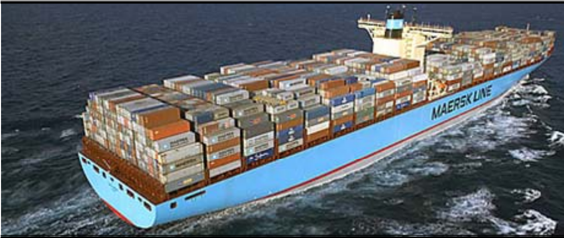
Figure 7: The “Emma Maersk”, an 11,000 TEU containership delivered in 2006 with a gross tonnage of 170,000 and 110,000 HP motor
