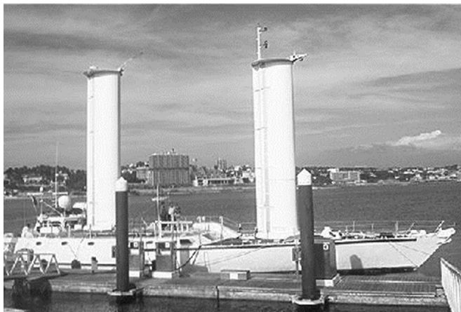
Fig. 4. Cousteau vessel Alcyone in harbor with its trademarked Turbosails propulsion system visibly dominant. (Source: https://commons.wikimedia.org/wiki/File:Rotorship_Alcyone_in_harbour.jp )
