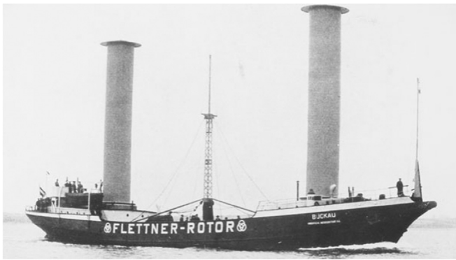
Fig. 2. First Flettner rotor ships Buckau (later renamed Baden-Baden ), circa 1925. (Source: http://www.deutsches-museum.de/en/information/young-people/inventors-trail/drivetrains/flettner-rotor/ )
