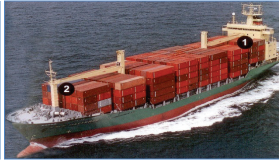
Fig.2b: Feeder vessel with on-board jib-crane source: Dokmar Maritime Publishers B.V. 6 th Edition.
