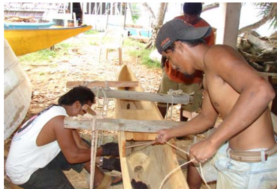
Figure 12: Lashing the hull of a canoe in progress. Photo credit Waan Aelōñ in Majeḷ
