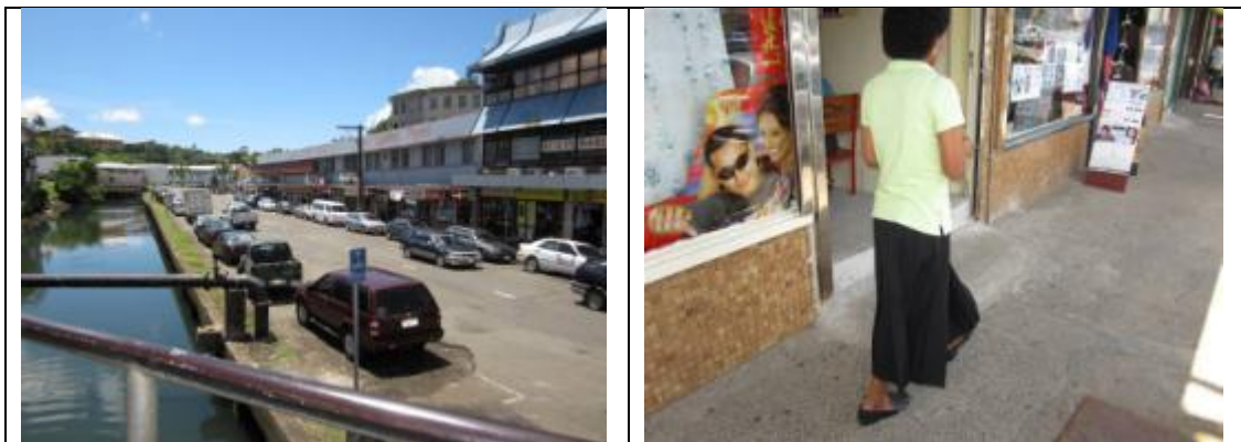
Photo1: At high tide Nabukalou Creek backs up and inundates the road and footpath adjacent to 8 shops in Greig Street at right of photo; Photo 2: Shops have steps to prevent entry of creek and flood water due to high tide and heavy rain.
