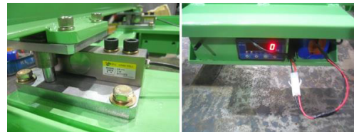
Fig.7 Load cell and Zigbee wireless communicating device
