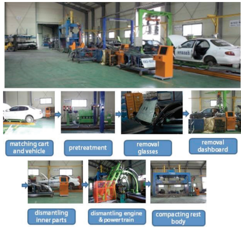
Fig.8 Implemented ELV dismantling stages
