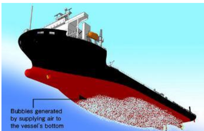
Figure 11: Hull air lubrication system
