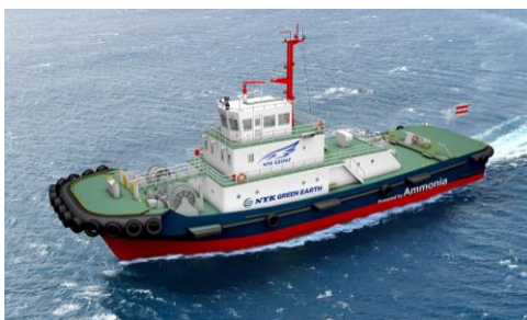
Figure 18: Tugboat reconfigured to run on ammonia
