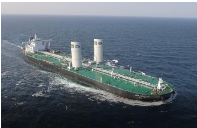
Figure 8: Rigid sails for large vessels
