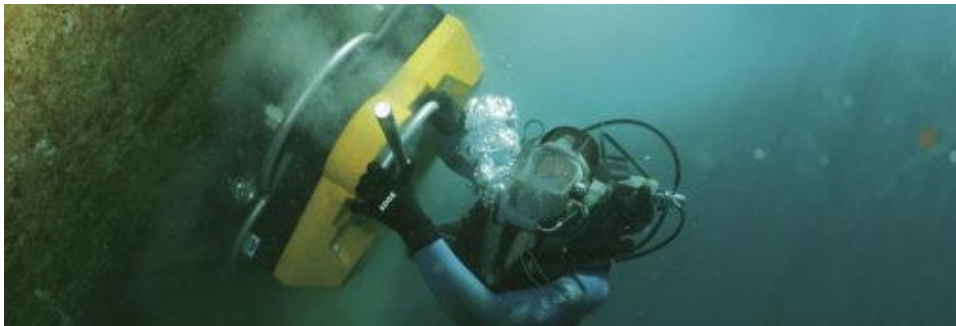
Figure 5: Diver performing underwater hull cleaning
